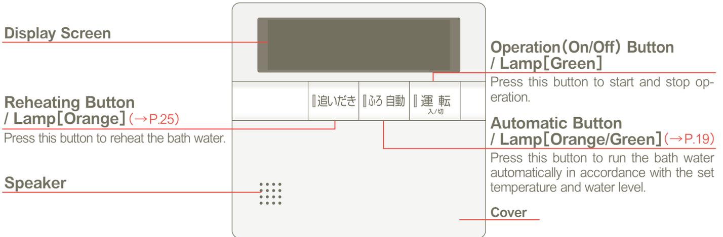
The following buttons are located inside the front cover of the kitchen remote controller.
